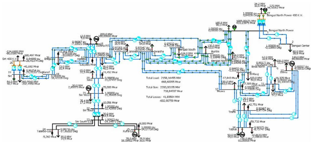
Fig. 3 Power flow load in transmission power system of Libya
