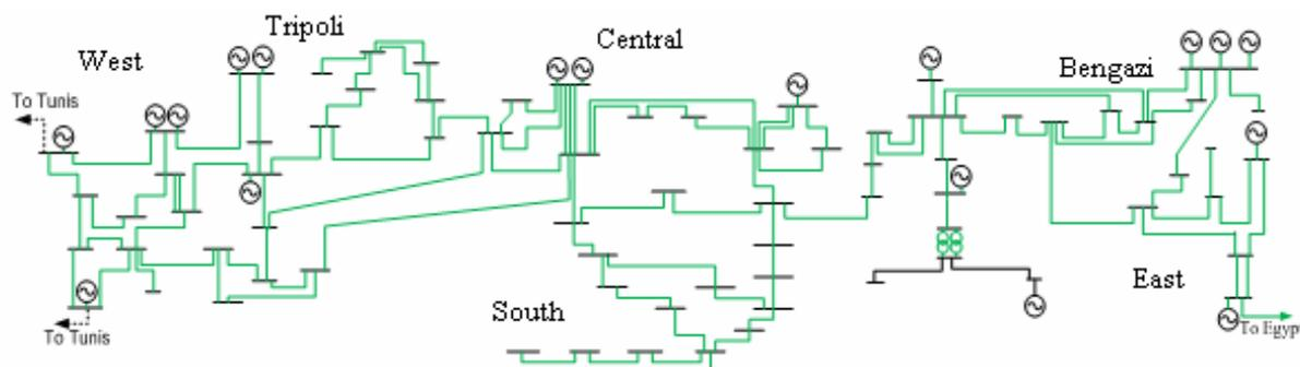
Fig. 1 Transmission power system of Libya
