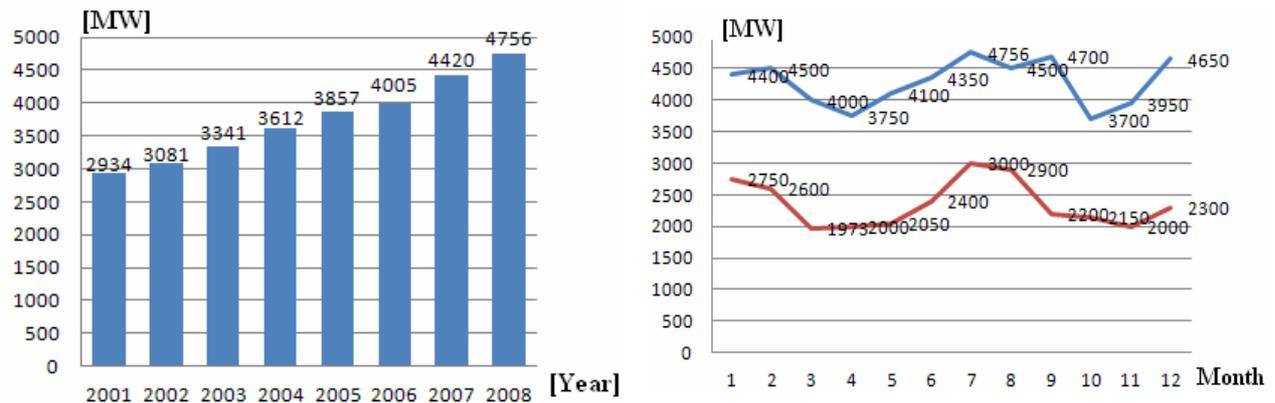
Fig. 2 Power load in transmission power system of Libya
