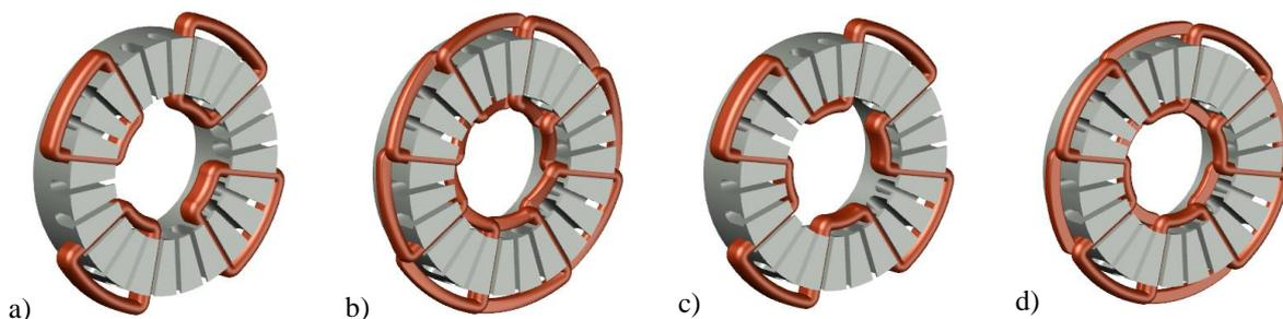
Fig. 1. Most common types of lap and wave windings.
