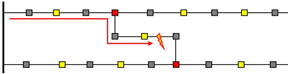
Fig.1 Failure management in the 22 kV cable network
