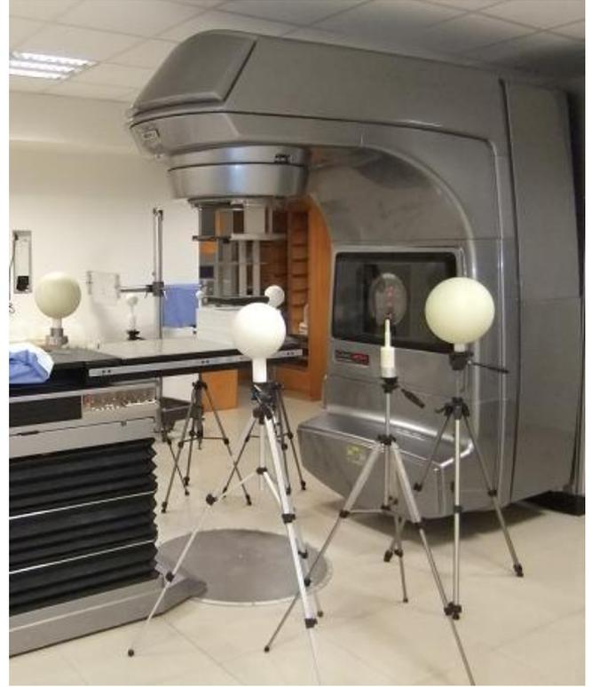
Figure 1. BSS/TLDs around the IC
