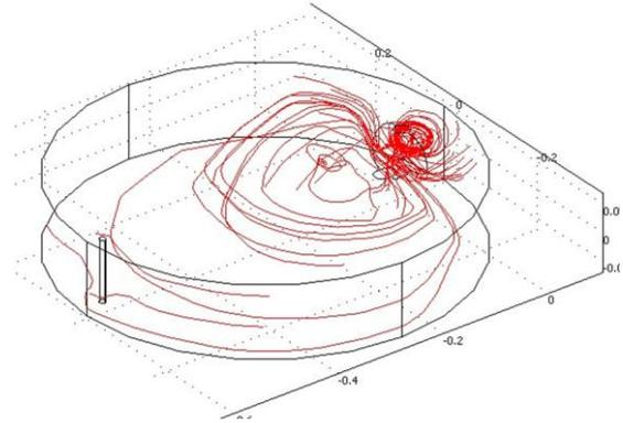
Figure 6. Magnetic flux density in streamlines at 100MHz
