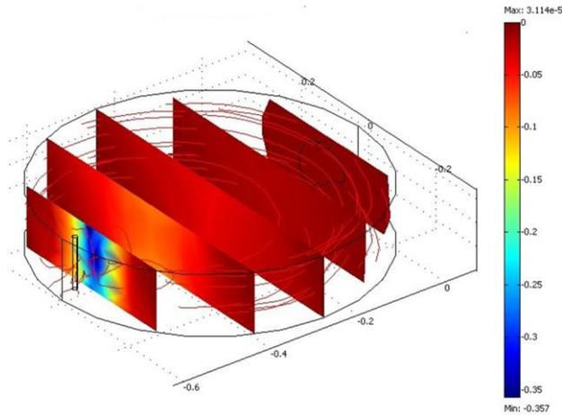
Figure 4. The slices are the electric field simulation. The streamlines are the magnetic flux density at 50 MHz
