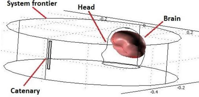
Figure 3. The brain is into the head model and the catenary is 50cm away from head. The extern cylinder define the system boarders
