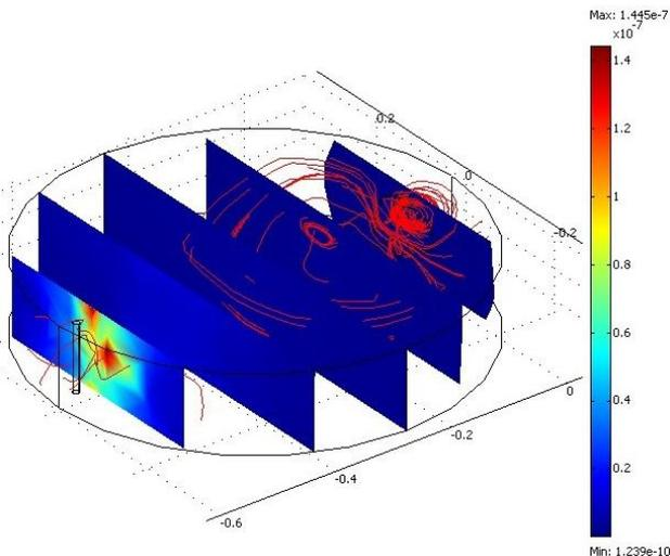
Figure 5. Magnetic flux density at 10MHz, showed in slices and stream lines
