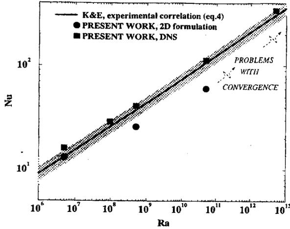
Figure 4: Prediction of Nusselt number in internally-heated fluid layers.
