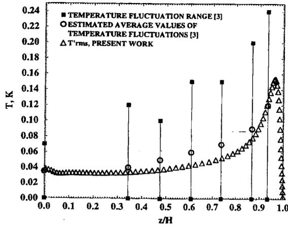
Figure 5: Temperature fluctuations: calculational results versus measurements.
