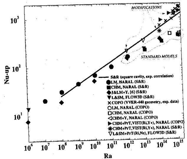
Figure 1: Variation of the average upwards  $Nu$  numbers with  $Ra$  numbers. Calculational results vs. experimental correlation of Steinberner and Reineke.
