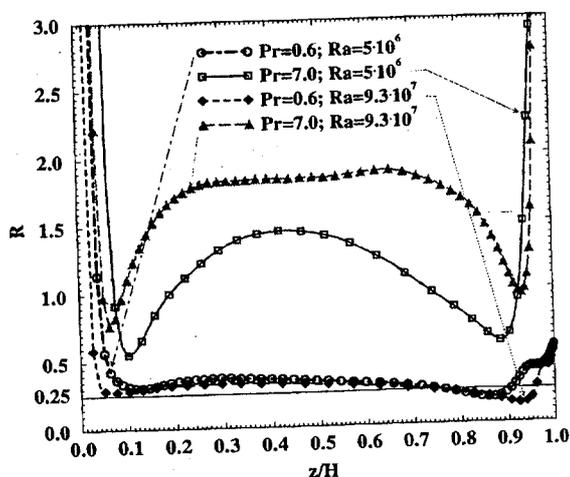
Figure 3: Dissipation time scale ratio  $R$  (proposed in RSM as constant, typically, in the range from 0.4 to 0.8).
