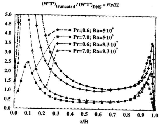
Figure 2: On applicability of the truncated algebraic form of the vertical turbulent heat flux (in case of validity, the ratio should be 1).
