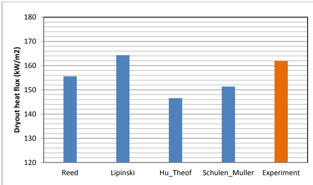
Fig. 12 Comparison of the dryout heat flux in Bed-2 with various models under top flooding conditions
