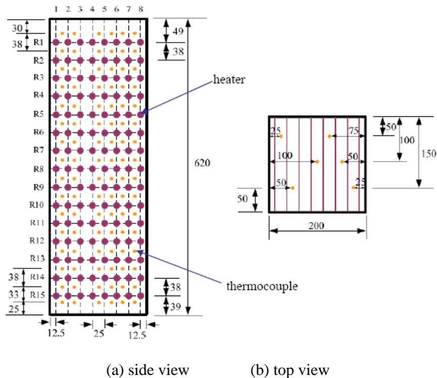
Fig. 8 Distribution of Heaters and Thermocouples
