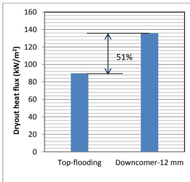
Fig. 11 Effect of downcomer on dryout heat flux in Bed-1
