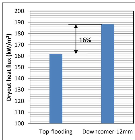
Fig. 13 Effect of downcomer on dryout heat flux in Bed-2
