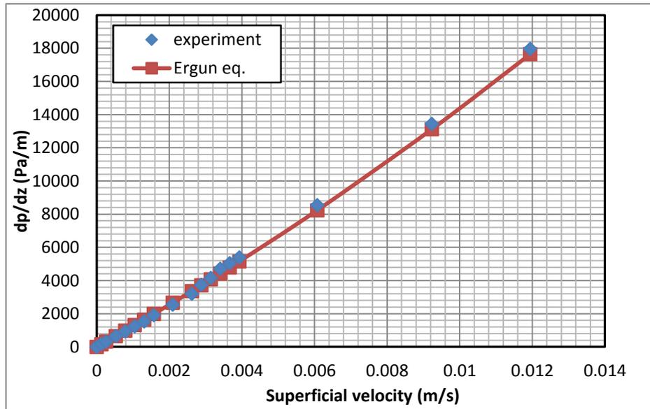
Fig. 6. Frictional pressure gradients of water flow in the Bed-2.
