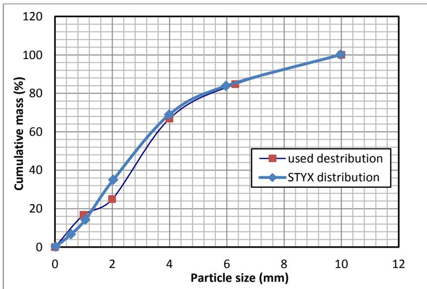
Fig. 4 Alumina gravels particle distribution (compared with Lindholm et al., 2006)
