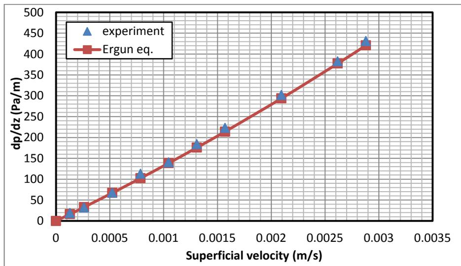
Fig. 2. Frictional pressure gradient of water flow in the bed packed with 3 mm single size spheres
