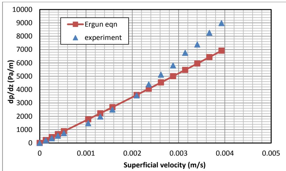
Fig. 5. Frictional pressure gradients of water flow in the Bed-1.
