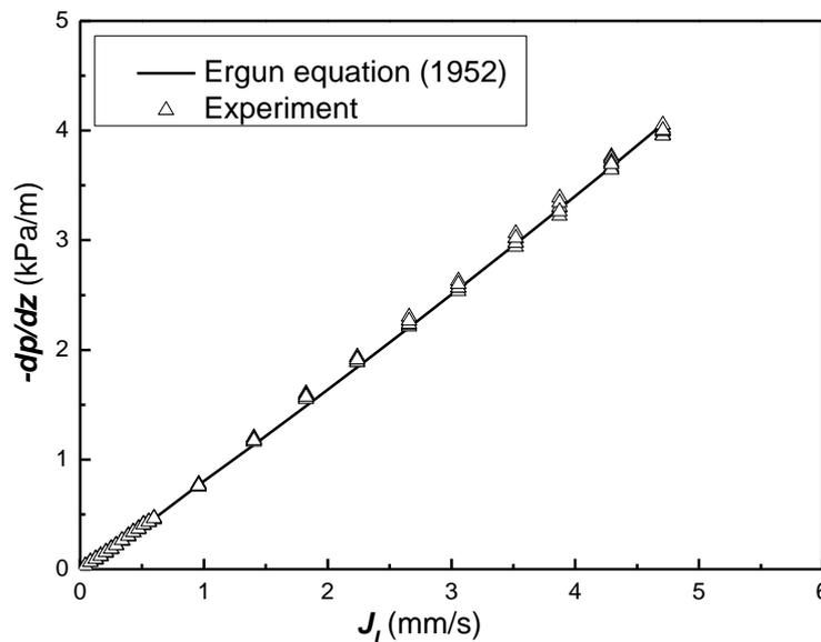
Fig. 9 Pressure gradients of water flow in the bed packed with 1.5 mm stainless steel spheres
