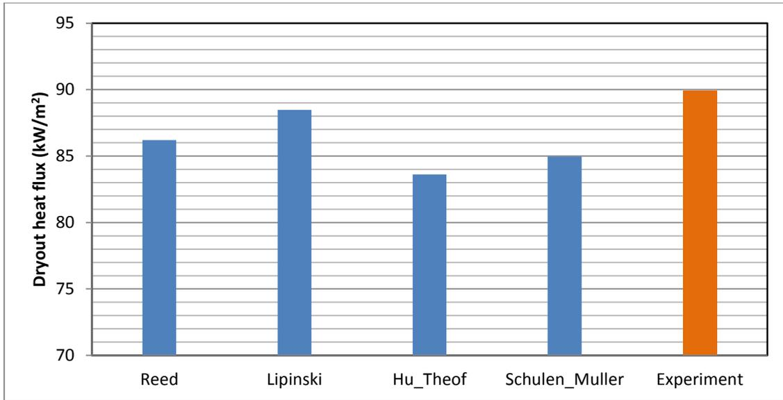
Fig. 10 Comparison of the dryout heat flux in Bed-1 with various models under top flooding conditions
