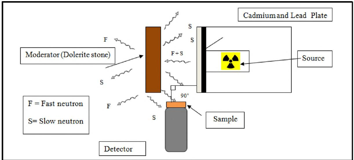
Figure 1: Thermal neutron test schematic diagram
