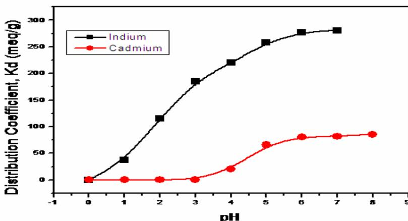
Figure (1): The effect of pH on the distribution coefficient of In(III) from Cd(II) by zirconium Vanadate.
