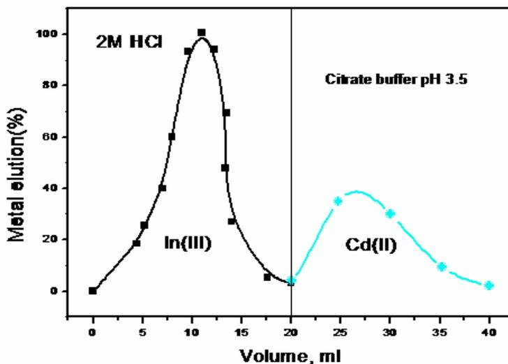
Figure (4): Elution curve of In(III) and Cd(II) onto zirconium vanadate using 2M HCl for indium and citrate buffer pH 3.5 for cadmium
