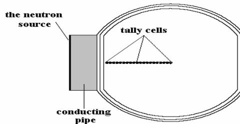
**Figure (3): The source-head assembly, showing the tally cells in brain region.**
