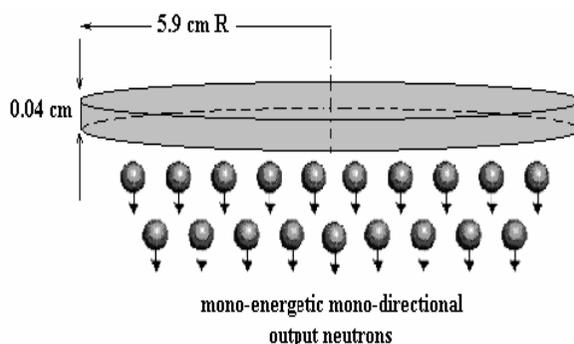
Figure (1): The neutron source.
