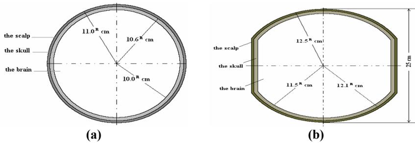
**Figure (2): The head model; (a) cross section, (b) and longitudinal section.**
