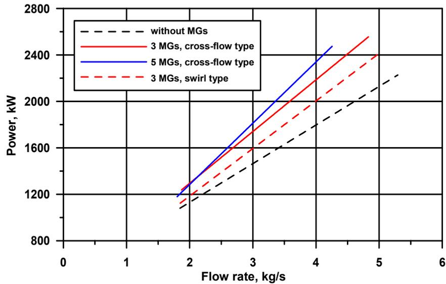
Figure 3 – Results of critical heat flux studies on the TVSA-ALPHA models with mixing grids (MG) (P = 15.7 MPa, T<sub>in</sub> = 290 °C)
