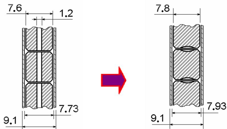
Figure 1 – Fuel rod design development to increase the fuel loading
