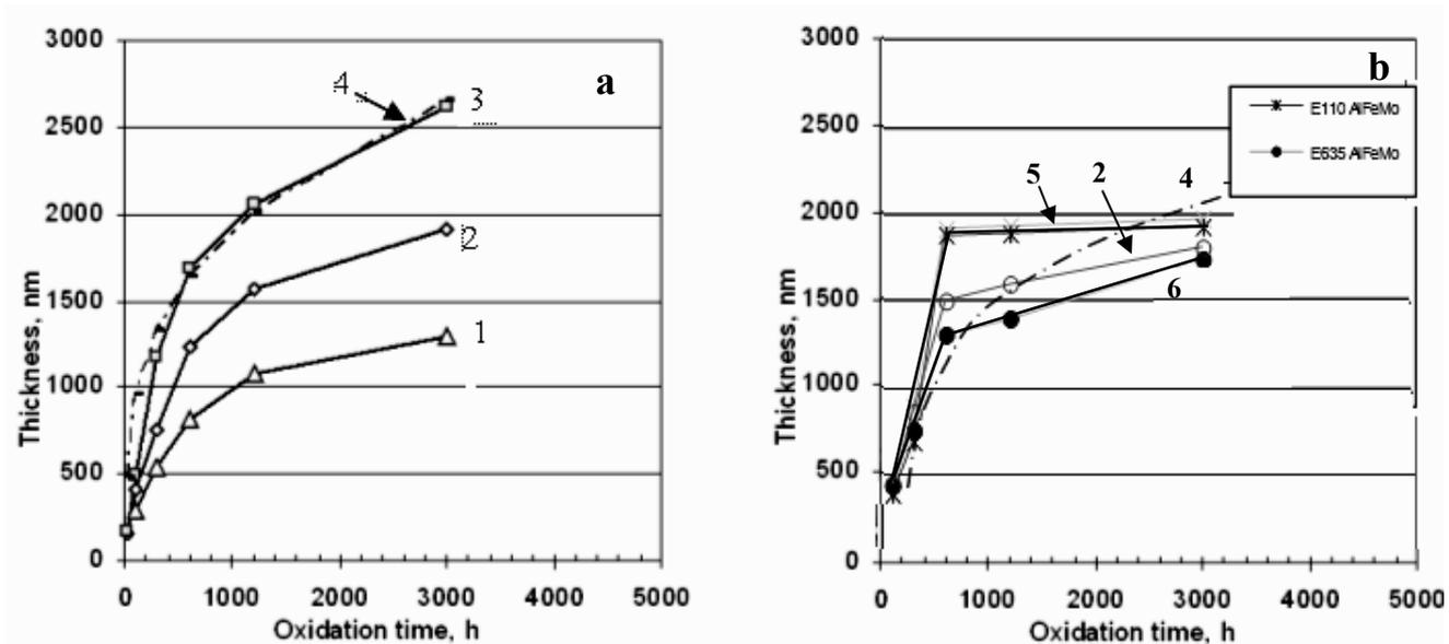
1 – Zr100, 2 – E110, 3 – E635, 4 –  $z(t) = a t^{0.33} + \text{const}$ , 5 – E110 alloying by MoFeAl atoms, 6 – E635 alloying by MoFeAl atoms
