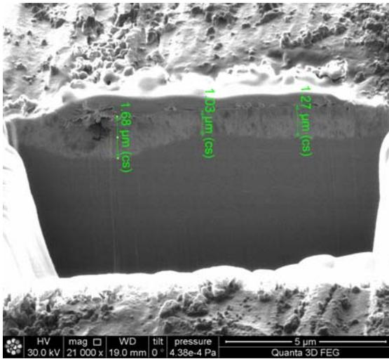
Fig. 2. Cross-section image of oxide films on a sample (smelting 5002) after oxidation for 300 h
