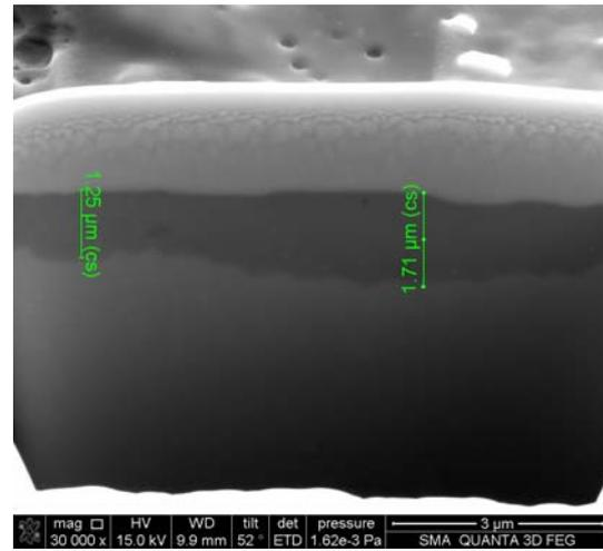
Fig. 3. Cross-section image of oxide films on a sample (smelting 5001/08) alloyed by the atoms of a Mo-Al-Fe three-layer film after oxidation for 300 h
