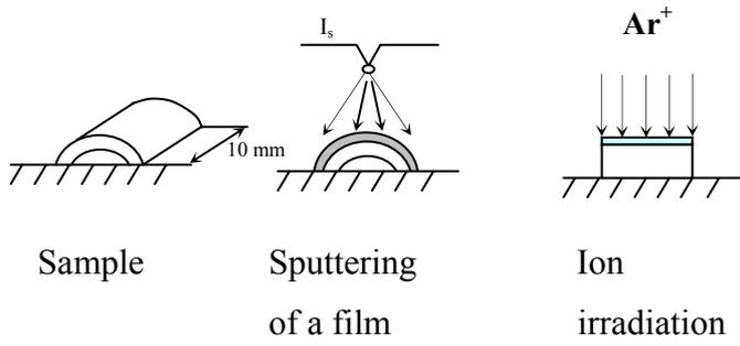
Fig. 1. A scheme of coating of a film onto the surface of a sample (using sputtering regime) and subsequent alloying by ion mixing under irradiation by  $\text{Ar}^+$  ions
