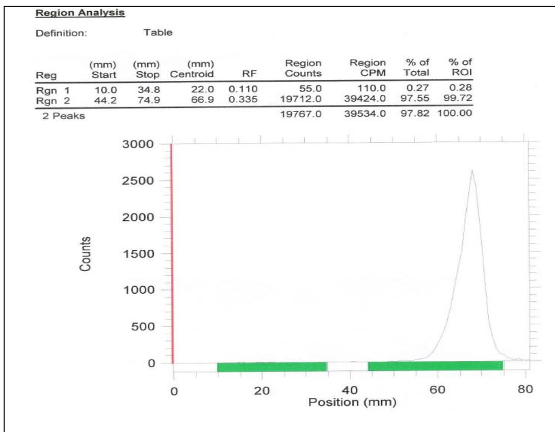
Figure 4: Chromatogram of radiochemical purity Tc 99m.
