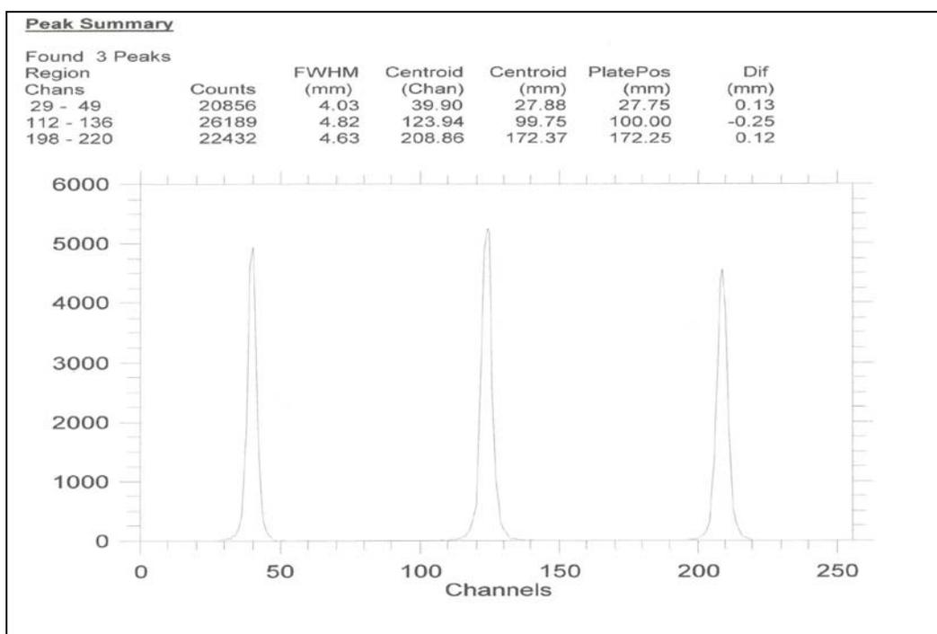
Figure 3: Chromatogram of Efficiency Calibration.
