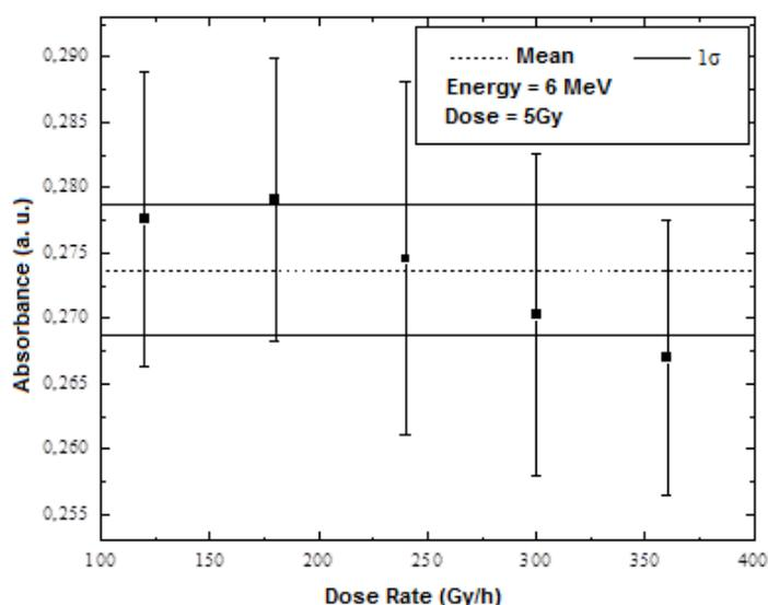
**Figure 3. Dose rate response of alanine gel solution to 6 MeV photon clinical beams radiation.**
