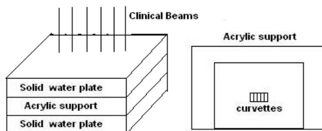
**Figure 2. Irradiation set up to photons electrons irradiations.**
