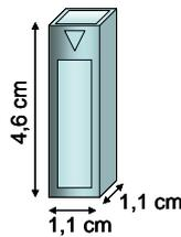
Figure 1. Cuvettes dimensions.
