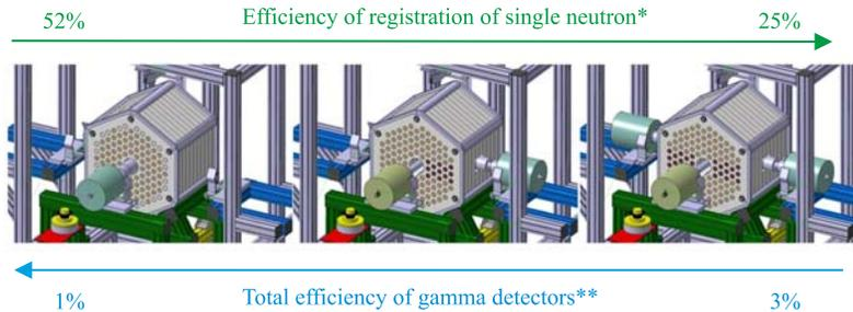
Fig. 3. Three available configurations to operate BEDO–Tetra installation. On the left-hand side — the  $1n$  is maximum, whereas efficiency of gamma registration is the minimum (experimentally measured values). On the right-hand side — the gamma efficiency is higher at the expense of  $\varepsilon_{1n}$  (calculated value). In the center — the transition configuration is presented. \* — for the 1 MeV neutron energy; \*\* — for the 1 MeV gamma energy
