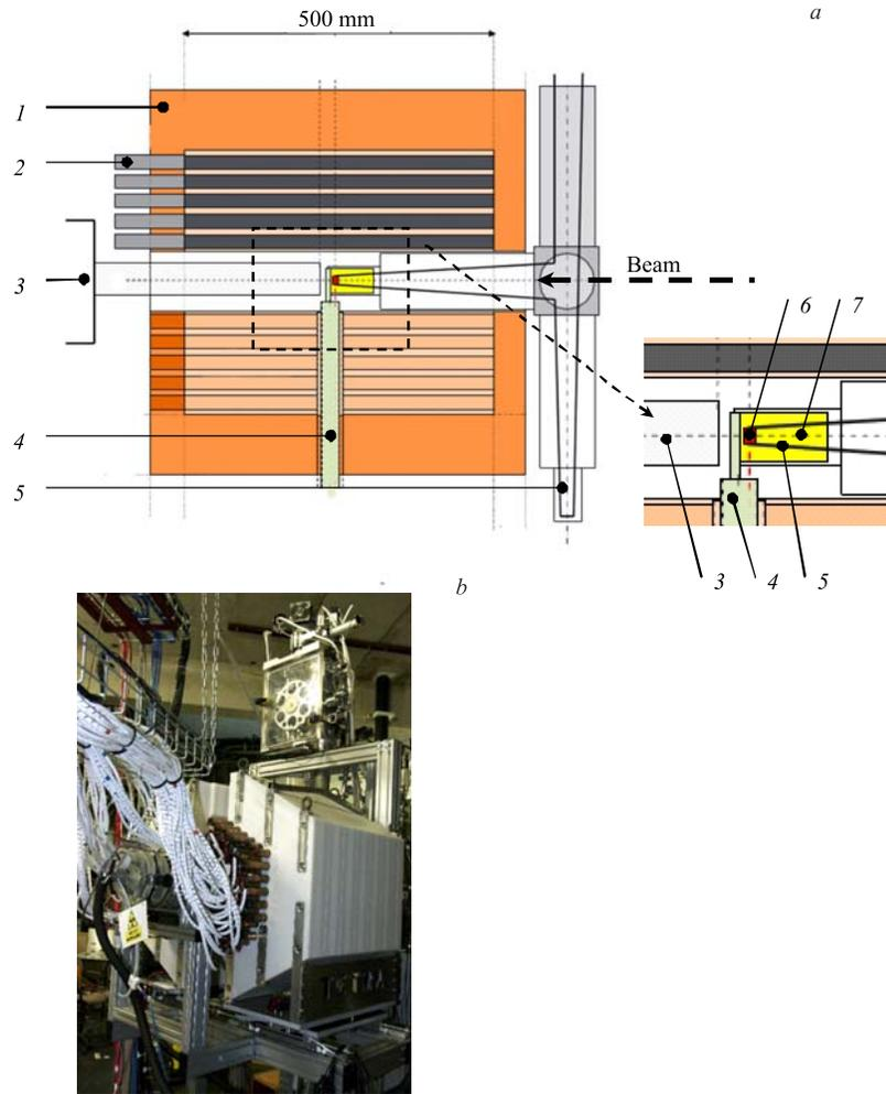
Fig. 2. The schematic view of TETRA setup (a): 1 — shielding borated polyethylene; 2 —  $^3\text{He}$  with preamplifier placed in moderator; 3 — germanium detector; 4 — light guide; 5 — tape; 6 — collection point; 7 —  $4\pi$  beta detector. The TETRA/BEDO installation (b)
