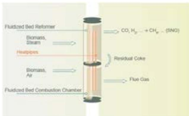
Figure 2 Picture of heatpipe-reformer [1]
