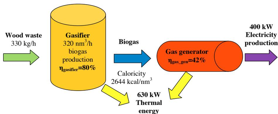
Figure 4 Thermal balances of the biomass installation [4]
