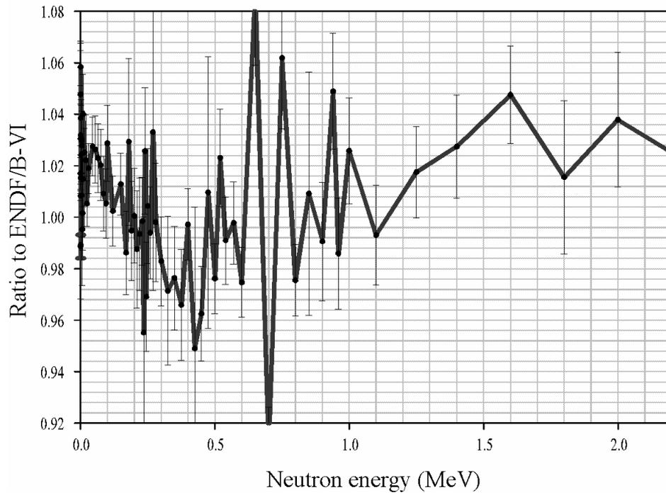
**Figure. 14 Comparison of the  $^{239}\text{Pu}(n,f)$  cross-section from this evaluation with the ENDF/B-VI evaluation**
