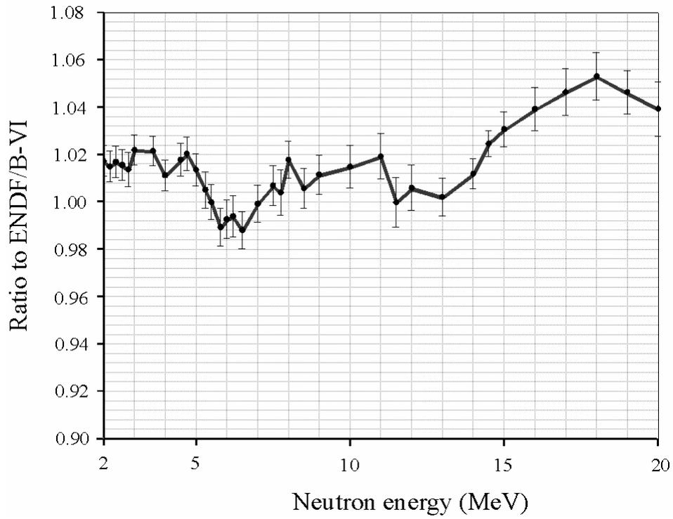
**Figure 12. Comparison of the  $^{238}\text{U}(n,f)$  cross-section from this evaluation with ENDF/B-VI evaluation up to 20 MeV and with updated values [23] above 20 MeV**
