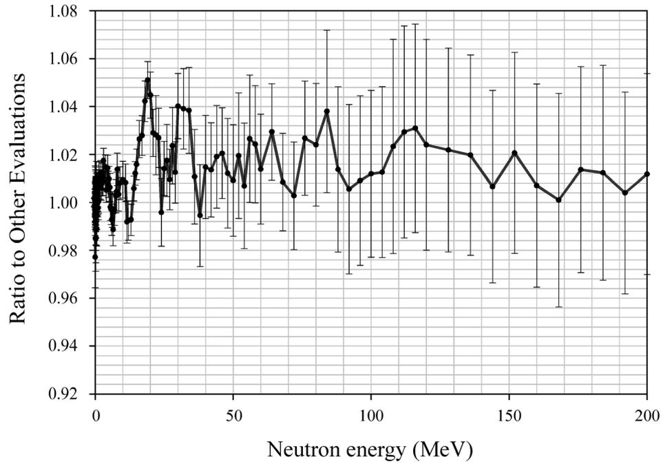
**Figure 11. Comparison of the  $^{238}\text{U}(n,f)$  cross-section from this evaluation with the ENDF/B-VI evaluation**
