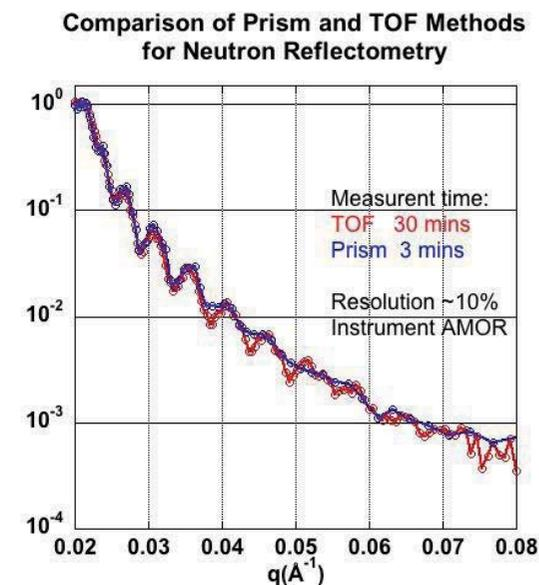
**Figure 2:** Reflectivity measured by the prism (blue) and TOF (red) methods. It was not possible to have the same resolution as a function of wavelength as AMOR operates with a constant  $d\lambda/\lambda$  like D17 and FIGARO in this case set at 10%. The prism produces a resolution with constant  $d\lambda$  which varies from about 5% at  $12\text{\AA}$  (corresponding to the lowest  $q$ ) to about 20% at  $2\text{\AA}$  (at the highest  $q$ ).
