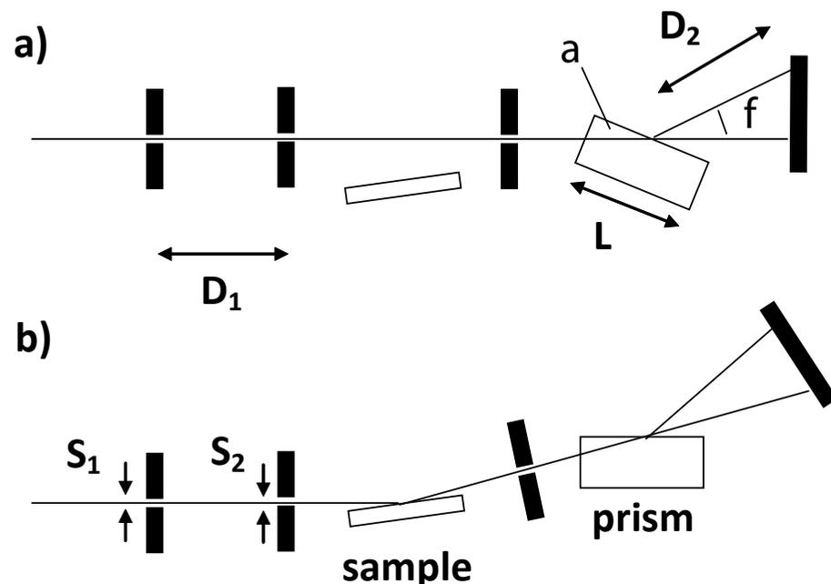
**Figure 1:** The experimental layout. The upper panel a) shows the experimental conditions for measuring the direct beam. The slit in front of the prism does not collimate the beam but simply ensures that all reflected neutrons pass through the prism.
