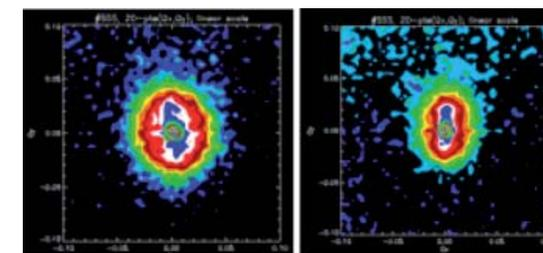
**Figure 3:** VCN-SANS plots for unstretched (left) and stretched (right) polymer blend.
