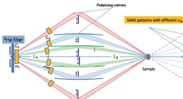
**Figure 2:** MIEZE encoding of multiple SANS RF flippers  $C_1$  and  $C_2$  are separated by  $L_1$  and produce time dependent signals at detector at  $L_2$  for frequency encoding.
