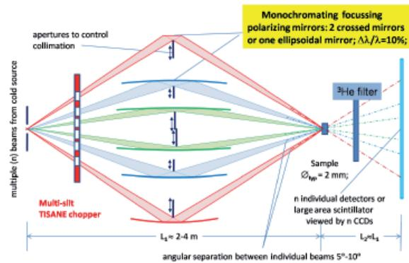
**Figure 1:** Focussing multiple SANS with multi-slit TISANE chopper for fast stroboscopic measurements.
