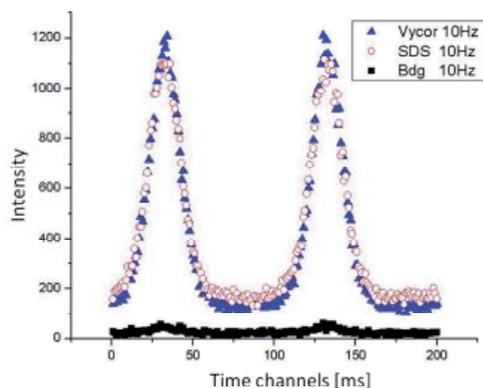
**figure 4:** Time dependent intensity at 10 Hz beam modulation, for Vycor (blue) and SDS micelles (red) and background (black).
