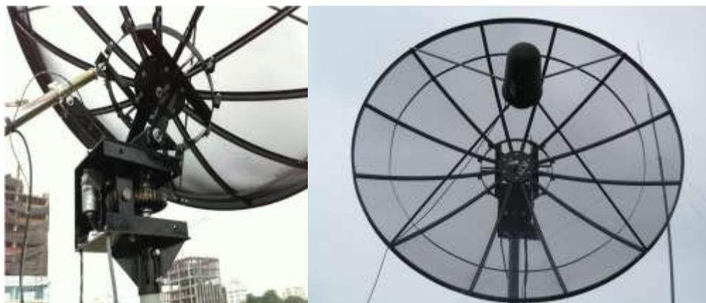
**Figure 1:** Close-up views of the SRT antenna and of the motor system (gear box and telescopic arm, left panel) and of the feed horn and the calibration antenna (right panel).
