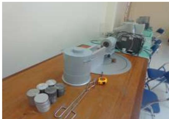
**Figure 1:** Compton scattering gamma measurement system at the Training Center, Nuclear Research Institute.
