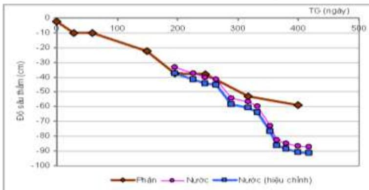
**Figure 5:** Infiltration of water and fertilizer on experiment time.
