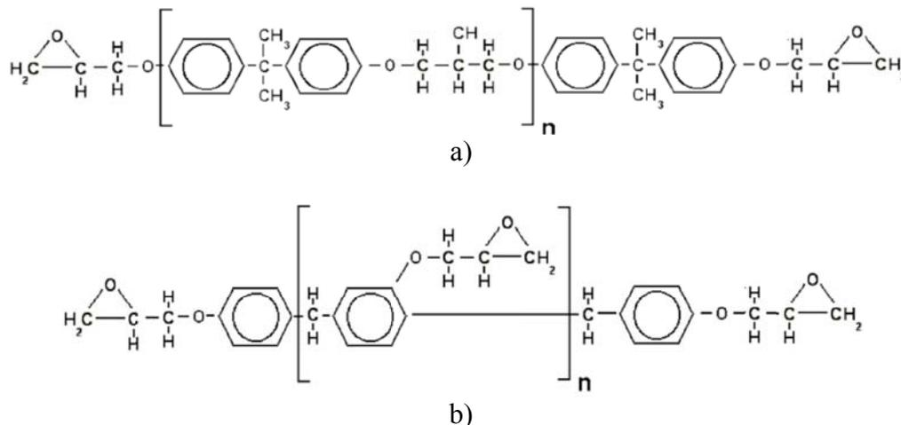
**Figure 1: Chemical structure of epoxy resins based on a) bisphenol A and b) bisphenol F.**
