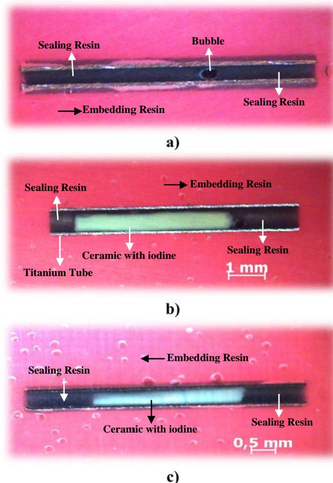
**Figure 3: Metallographic Images after sealing tests: a) Empty tube; b) Decentralized seed and; c) Centralized seed.**
