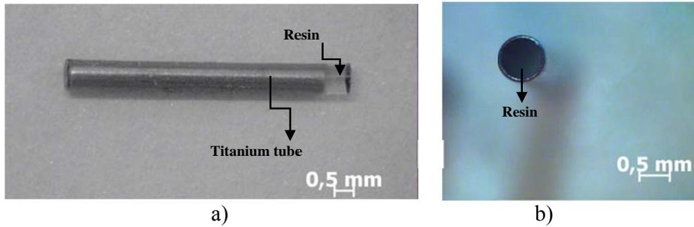
**Figure 2: Titanium tubes filled with resin: a) Aspect of the resin; b) Sealed tube.**
