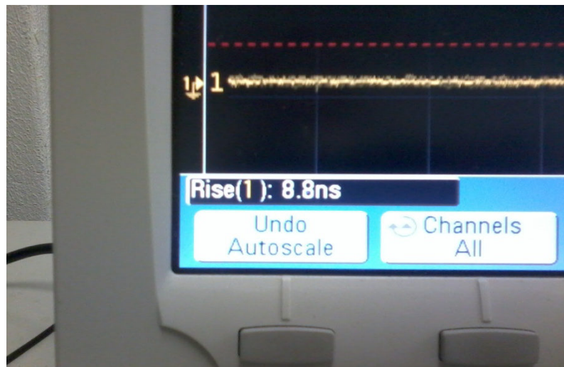
Figure 3: Detail of the PSC risetime measurement.
