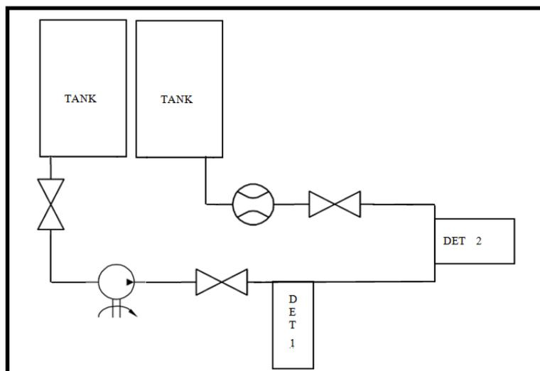
**Figure 2.1: layout of transport line to organic compounds installed in the laboratory.**
