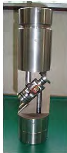
Inside picture of stress meter for horizontal and inclined components
