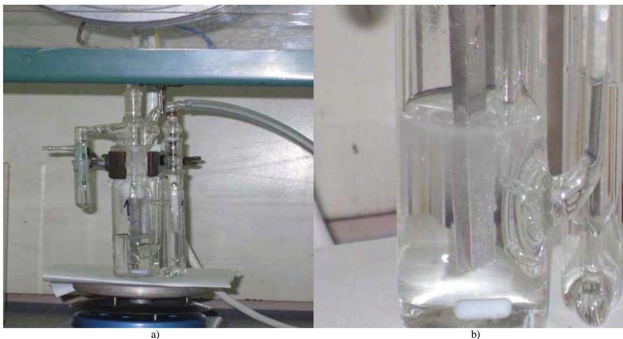
Fig.3. The electrolytic cell completed in Laboratory for radioisotopes, Institute “Vinča” (a) and electrolytic separation of gas  $\text{H}_2$  (b).
