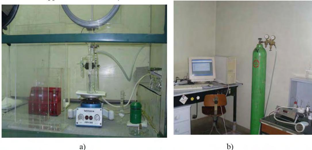
Fig.1. The equipment for electrochemical separation (Laboratory for radioisotopes, Institute “Vinca”) (a) with supplying of argon gas (b)
