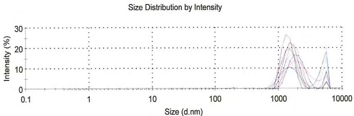
Fig. 1: The size distribution of synthesized HAp particles (PCS method)
