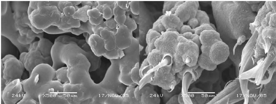
Fig. 2: SEM pictures of macroporous PE and GMA grafted PE
