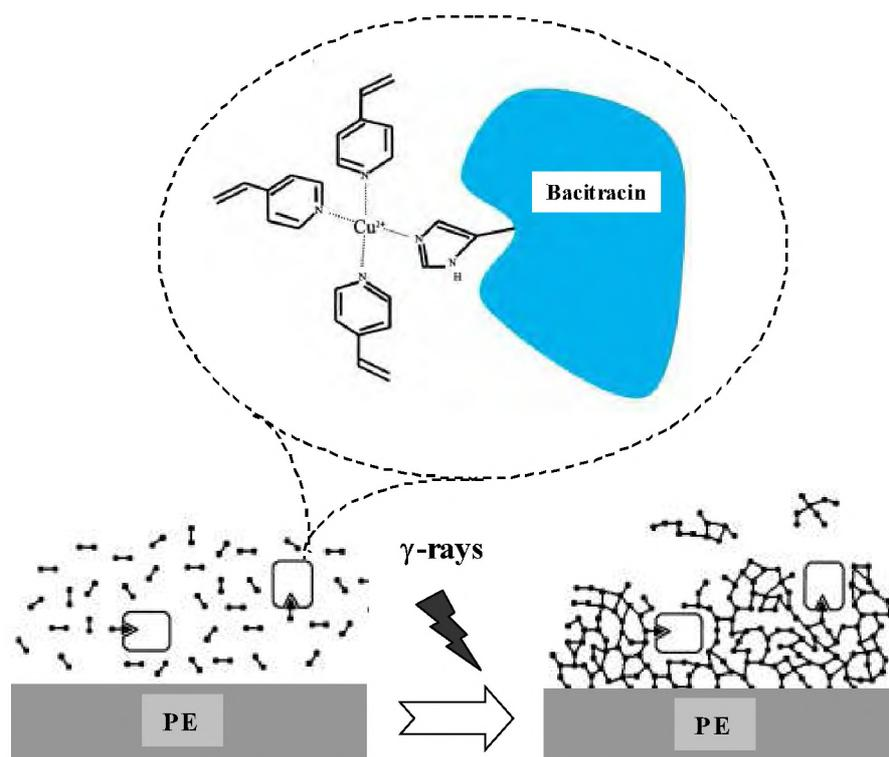
**Fig. 1:** Scheme of simultaneous imprinted surface grafting of PE by gamma rays in an aqueous solution
