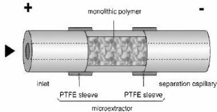
**Fig. 4:** Schematic representation of the monolithic microextractor into a capillary electrophoretic column
