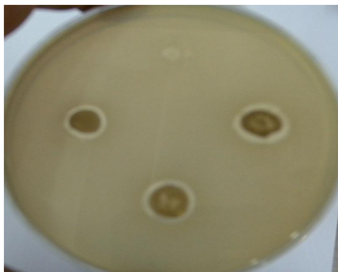
Fig. 5. The biological properties of Ag-CA nano composite of different silver contents towards gram negative bacte
