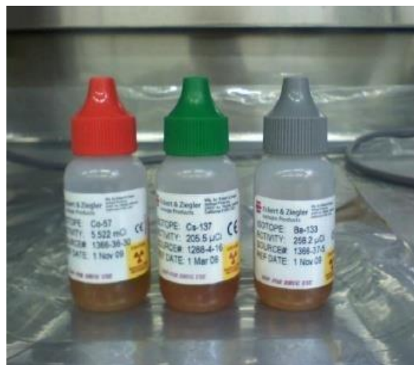
Figure 2: Sealed radioactive sources produced with cobalt-57, cesium-137 and barium-133. [2]
