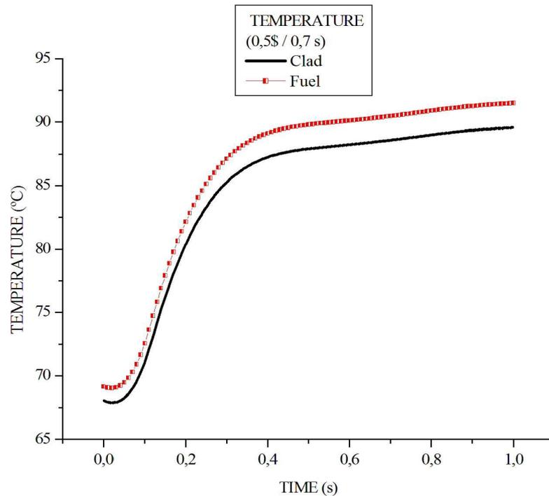
**Figure 6: Transient of Temperature for 0.5 / 0.7s inserted externally.**
