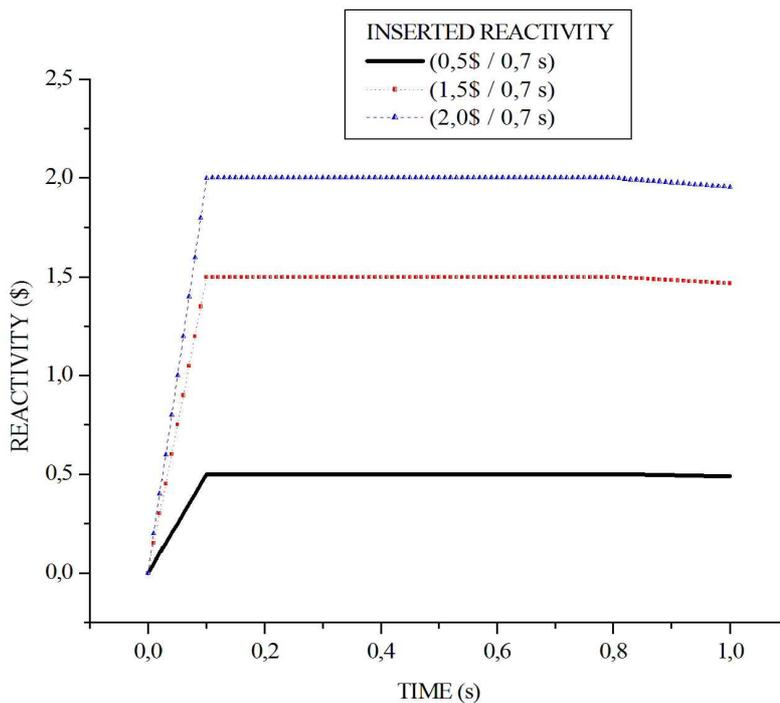
**Figure 3: Reactivity externally inserted IAE-R1.**
