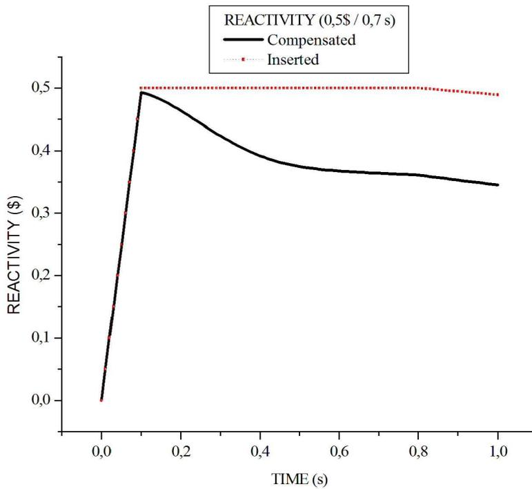
**Figure 5: Transient of the reactivity of \$ 0.5 / 0.7s and externally inserted.**
