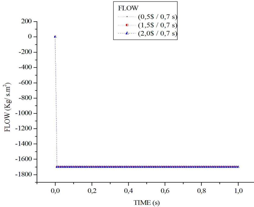
**Figure 4: Transient of the inlet mass velocity.**
