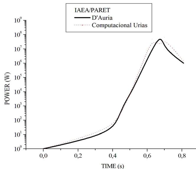
**Figure 2: Validation of the power profile with IAEA generic reactor [6].**
