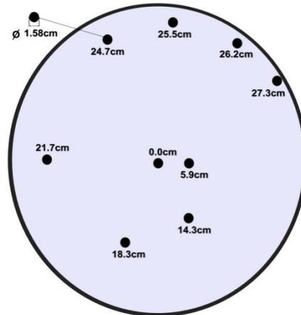
**Figure-4: Top view of the drum indicating the position of the sources**
