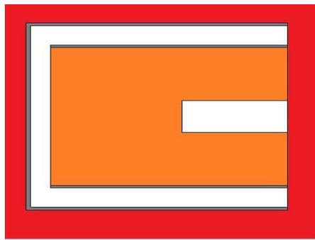
**Figure-2: Lateral view of the detector. Orange color: Ge crystal; grey color: aluminum; white color: vacuum; red color: air.**
