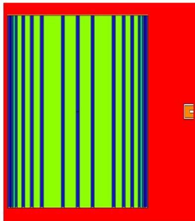
**Figure-3: Longitudinal view of the complete experimental setup, showing the position of the detector and location of radioactive sources. Orange color: Ge crystal; grey color: aluminum; white color: vacuum; red color: air; blue color: mixed source of  $^{152}\text{Eu}$  and  $^{241}\text{Am}$ ; green color: compressed paper.**
