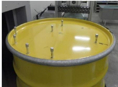
**Figure-1: Calibration drum filled with compressed paper positioned on the moving platform and mixed sources of  $^{152}\text{Eu}$  and  $^{241}\text{Am}$ .**
