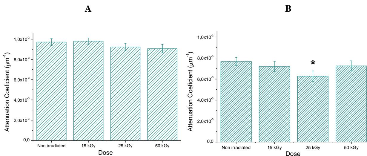
Figure 2: A) Graphs of the optical attenuation coefficients of the frozen, non irradiated samples and those irradiated with doses of 15, 25, and 50 kGy. B) Graphs of the optical attenuation coefficients of lyophilized, non irradiated samples and those irradiated with doses of 15, 25 and 50 kGy. (\*) indicates the difference, statistically, significant related to the control.
