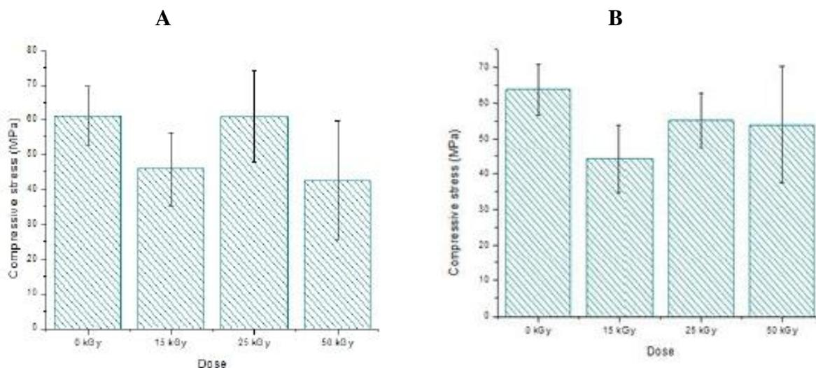
FIGURE 3 – **A)** Graph of the compressive stress mean, at the moment the sample breaks (MPa), frozen non irradiated and irradiated with doses of 15, 25 e 50 kGy. **B)** Graph of the compressive stress mean, at the moment the sample breaks (MPa), lyophilized non irradiated and irradiated with doses of 15, 25 e 50 kGy.
