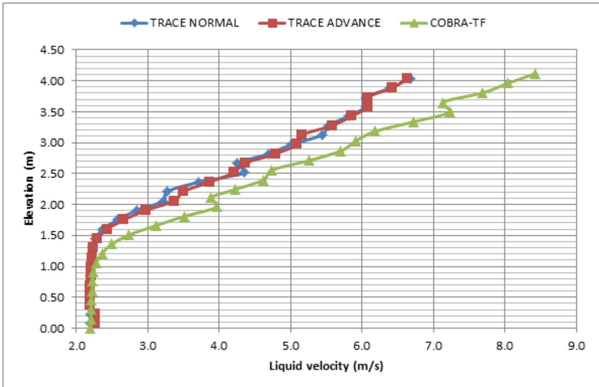
Figure 10: Comparison of the axial profile of liquid velocity.
