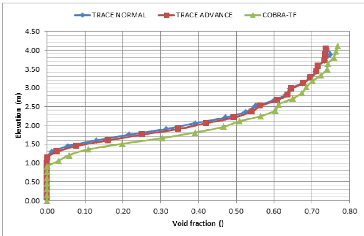
Figure 7: Comparison of the void fraction axial profile.
