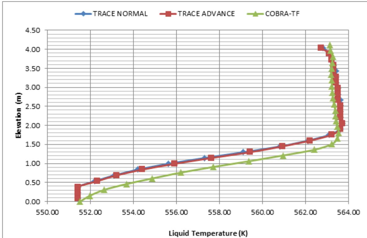
**Figure 8: Comparison of the axial profile of liquid temperature.**
