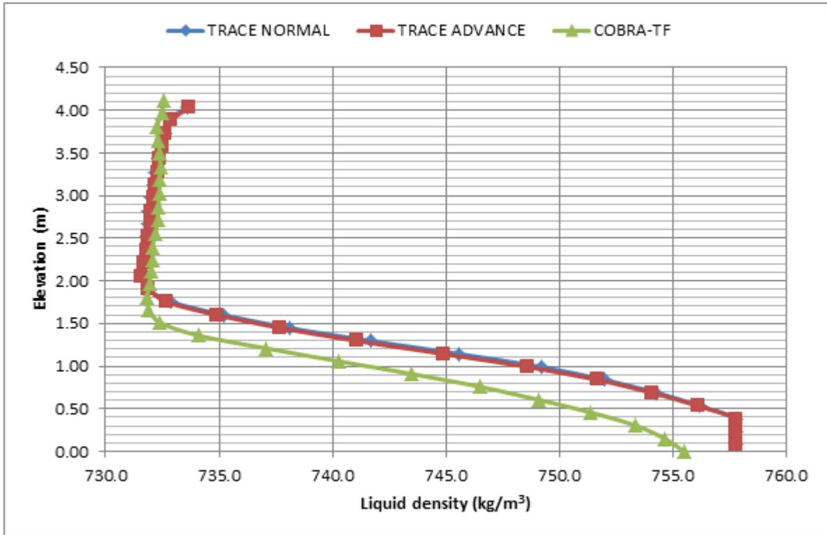
Figure 9: Comparison of the axial profile of liquid density.
