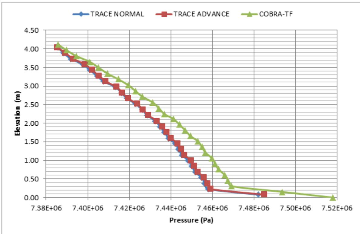
Figure 6: Comparison of pressure drop axial profile.
