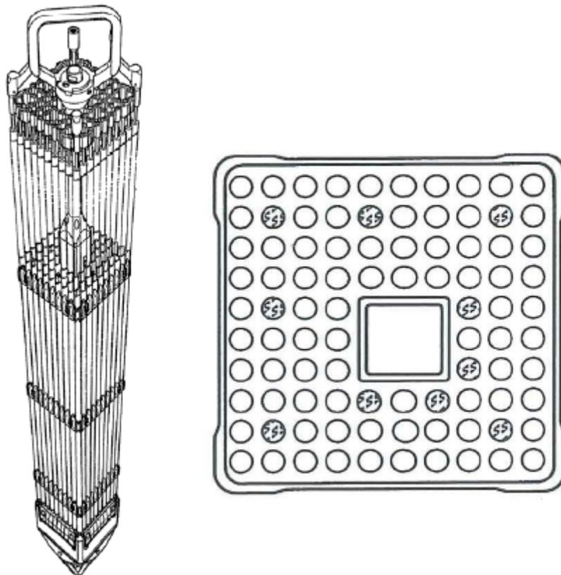
**Figure 1: Scheme of the analyzed 10x10 BWR fuel assembly.**
