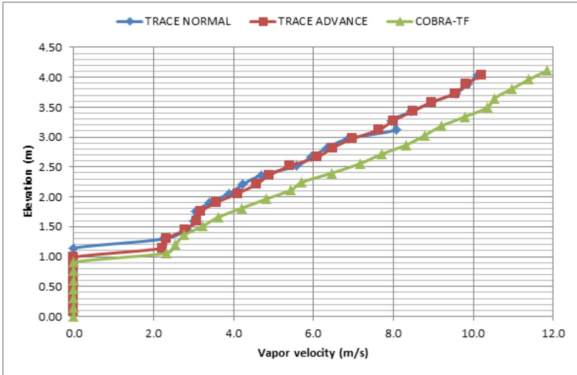
Figure 11: Comparison of the axial profile of vapor velocity.
