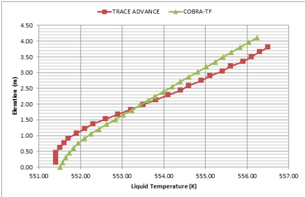
Figure 12: Comparison of the axial profile of liquid temperature in the water rod.
