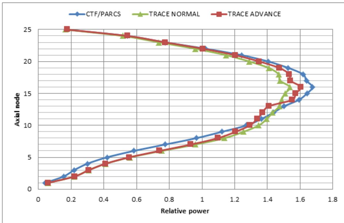
**Figure 5: Comparison of the axial power profile.**
