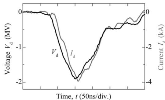
Fig.7 Typical waveforms of voltage and current at the diode
