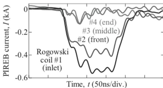
Fig.4 PIREB current in treatment chamber at various positions
