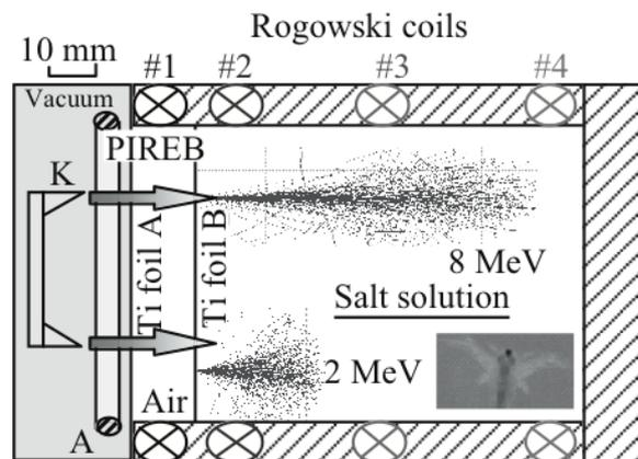
Fig.2 Side view of treatment chamber. Calculated electron trajectories are also indicated
