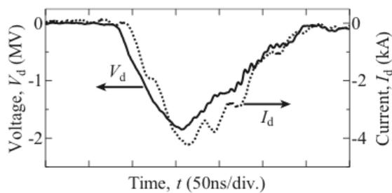
Fig.3 Typical voltage and current waveforms at diode
