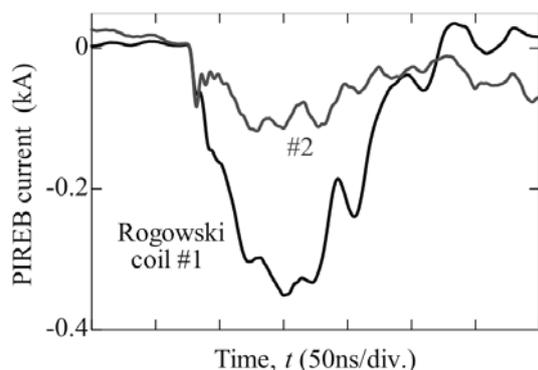
Fig.8 Typical waveforms of PIREB current detected at each Rogowski coil as shown in Fig.6
