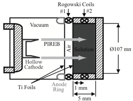
Fig.6 Experimental setup of PIREB irradiation of a reactor containing a congo red solution
