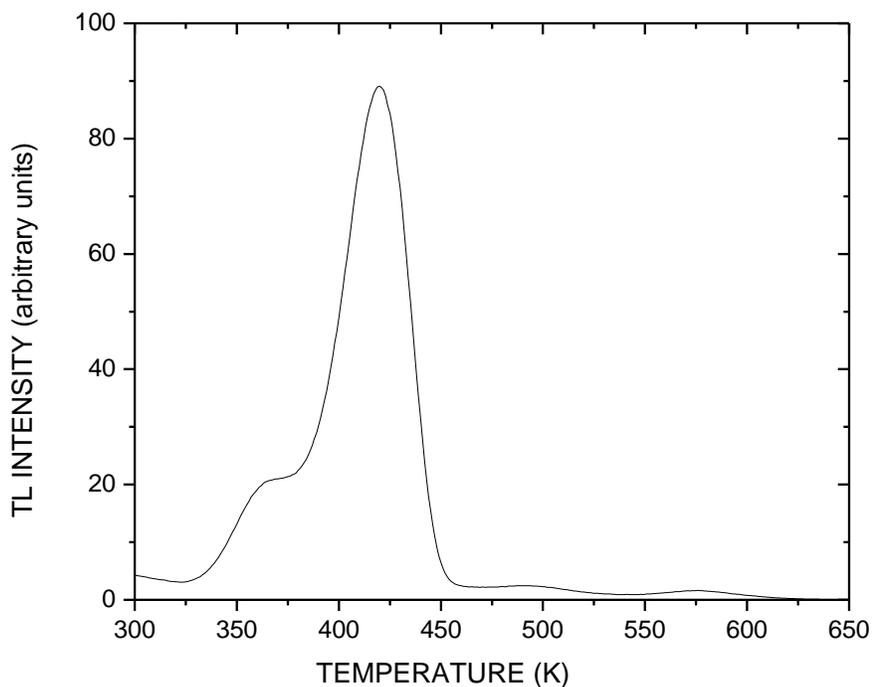
*Figure 1.- Glow curve of a ternary crystal thermally treated sample after being exposed to beta ray irradiation.*
