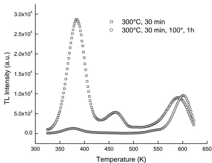
*Fig. 3.- TL curves heat treated at 573K (300° C), 30 min in the first one and 573 K 30 min then released 1 h at 373 K in the second one.*
