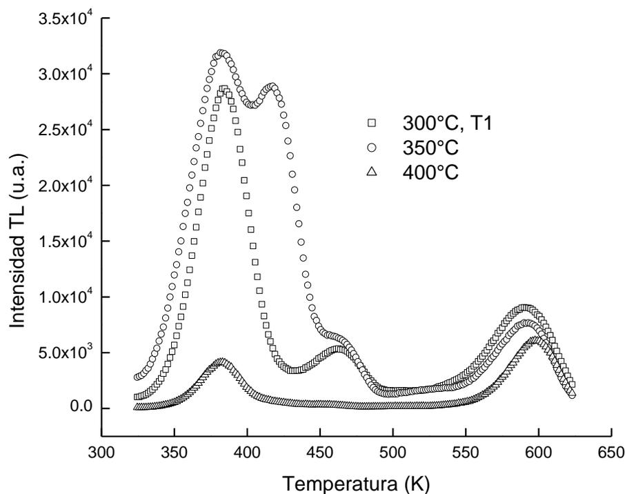
Figure 2.-Glow curves of the samples subjected to different heat treatments
