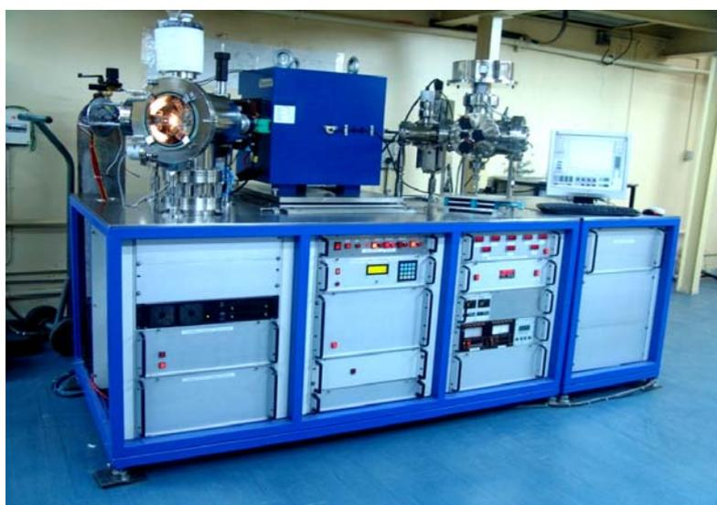
Fig. 1. Photograph of the latest version of indigenous TIMS Instrument
