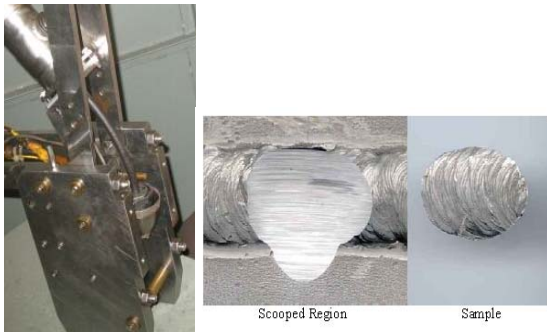
Fig. 1: Scooping device, scooped region and scooped sample
