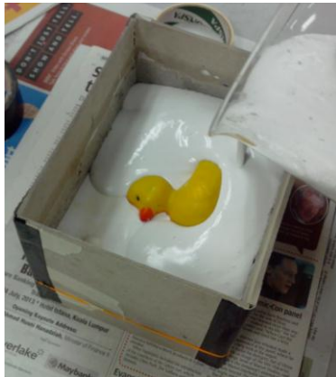
6) The plaster slurry poured on the first mold.
