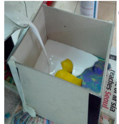
4) The mixed plaster and water poured on molding sand.
