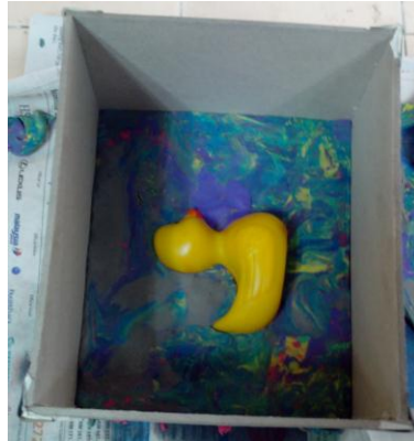
2) Molding sand as base and cover half part of masterpiece.
