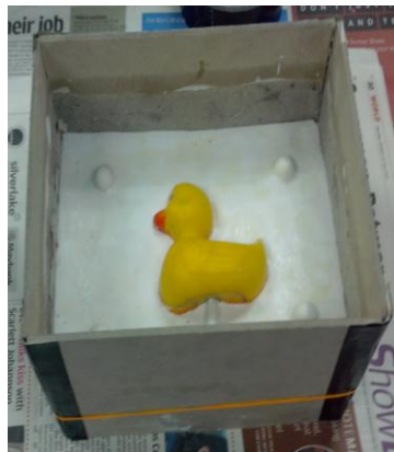
5) The first half moulding mold inverted and molding sand removed.
