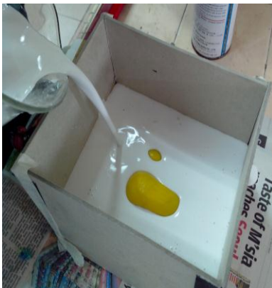
7) The plaster slurry poured to produce second mold.
