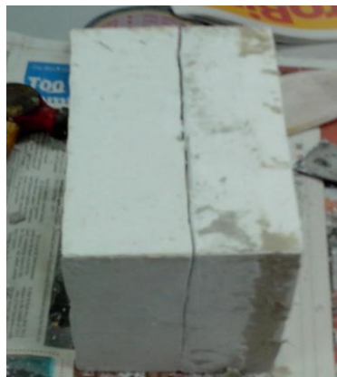
8) The mold is ready to separate and de-molded.
