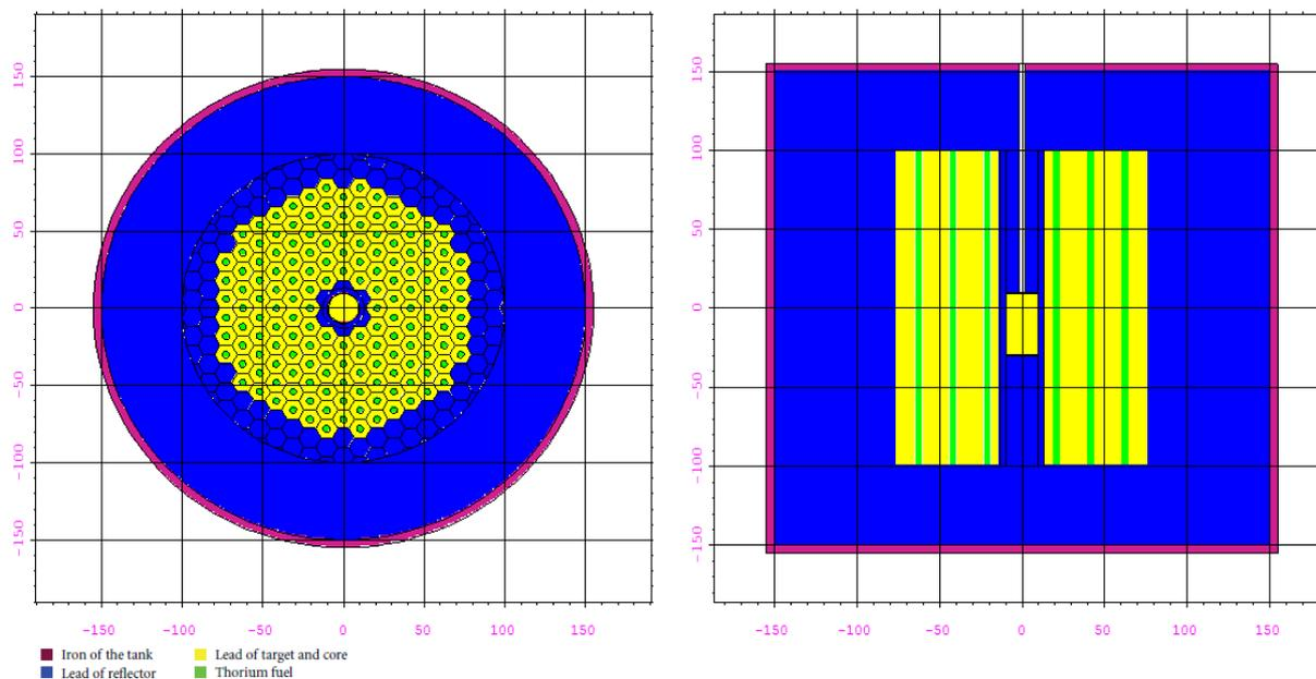
**Figure 1: Horizontal and vertical cross sections of the ADS.**
