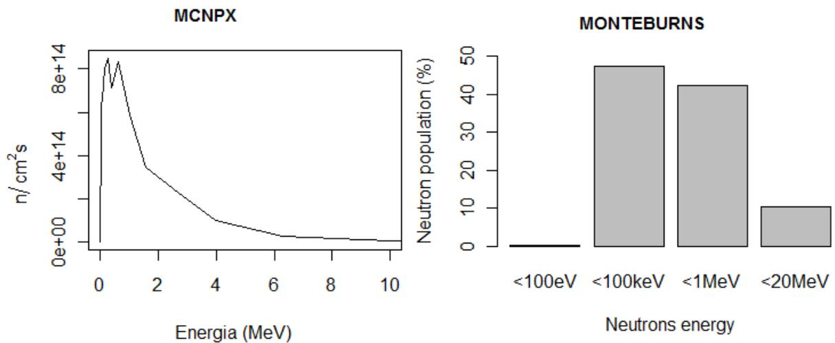
**Figure 3: Neutron spectra in the beginning of life.**
