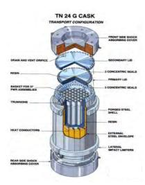
The advantages are modularity, high capacity, passive cooling and dual purpose storage and transport capability.
