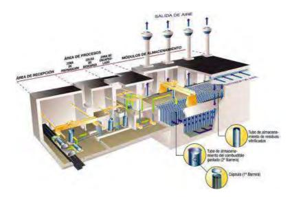
The concept will be implemented in the Spanish ATC (see picture): here, small canisters (typical capacity 6 UNF) are stored in a protected building with natural convection cooling. Both types of canisters can be stored (vitrified fission products UC generated by recycling or canisters containing UNF).
