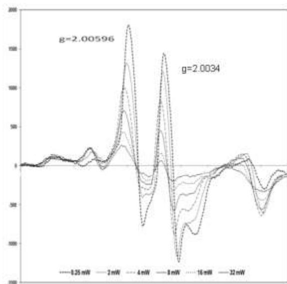
Fig 6 EPR spectra of a sample irradiated with 5 MeV electrons with a dose of 6.5 MGy at different microwave power
