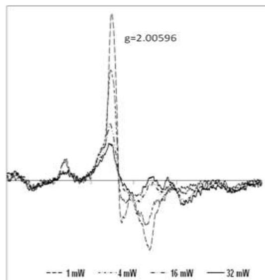
Fig 7 EPR spectra of a sample irradiated with 290 MeV/u Carbon beam with a dose of 1.5 kGy at different microwave power.
