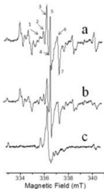
Fig.1 EPR spectra for samples irradiated with a) 5 MeV electron beam; b) gamma radiation and c) 290 MeV/u Carbon beam.
