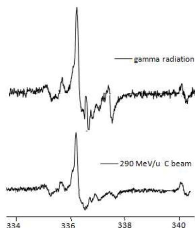
Fig.2 EPR spectra for samples irradiated with a) gamma radiation and b) 290 MeV/u Carbon beam with a dose of 1.5 kGy.
