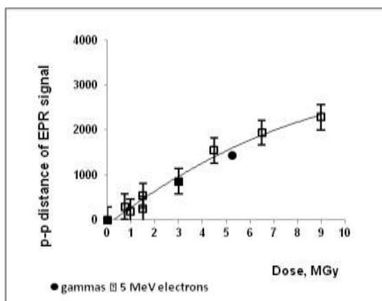
Fig 5 EPR signal intensity in arbitraries units for the peak 5 in a sample irradiated with electron beam
