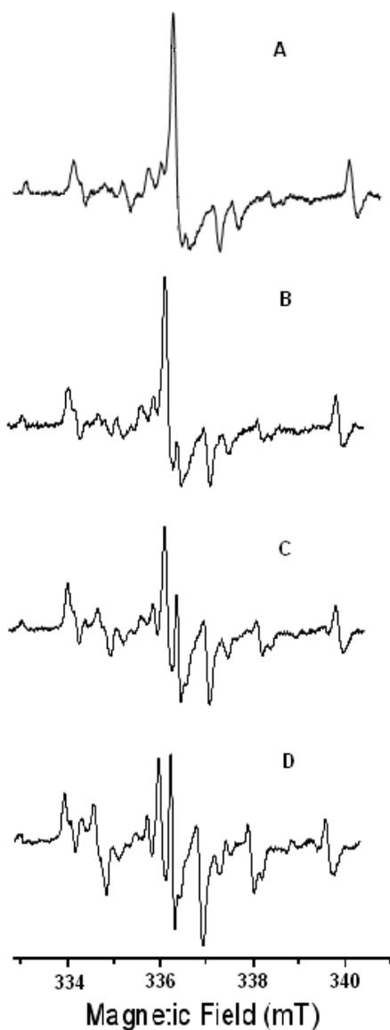
Fig. 3 Effect of the irradiation dose in the EPR spectra of calcium Carbonate irradiated with 5 MeV electron beam. Legend A= 0.74 MGy, B=1.5 MGy, C=6.5 MGy and D=9 MGy.
