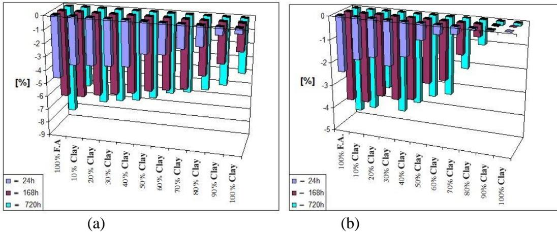
Figure 4. Leaching of the composites in acid medium (0.1MHCl) a. composites sintered at 1050<sup>0</sup>C, b. composites sintered at 1100<sup>0</sup>C
