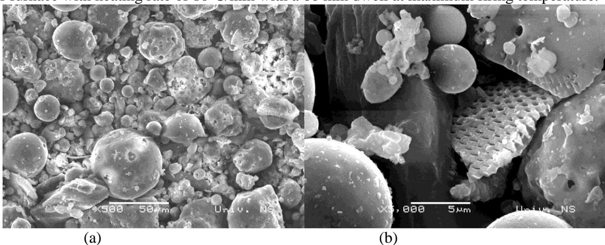
Figure 1. Morphology of the fly ash (a). bar 50µm, (b). bar 5 µm
