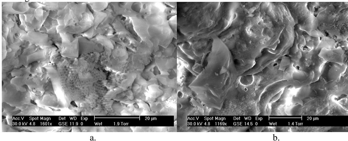
Figure 5. Microstructures of composites with 40wt.% fly ash content (bar 20µm) a. sintered at 1050<sup>0</sup>C
