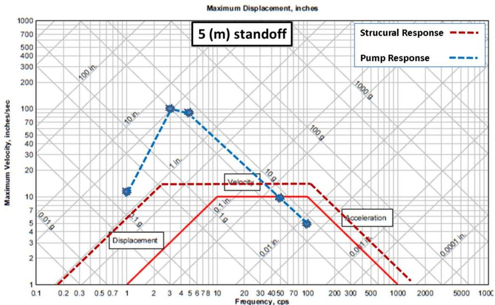
Figure 3. Pump fragility versus in-structure shock spectra due to external 100 kgs. TNT exploding 5 meters from the structure
