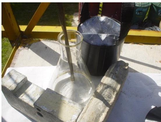
Figure 3. Preparation setup of tracer solutions.
