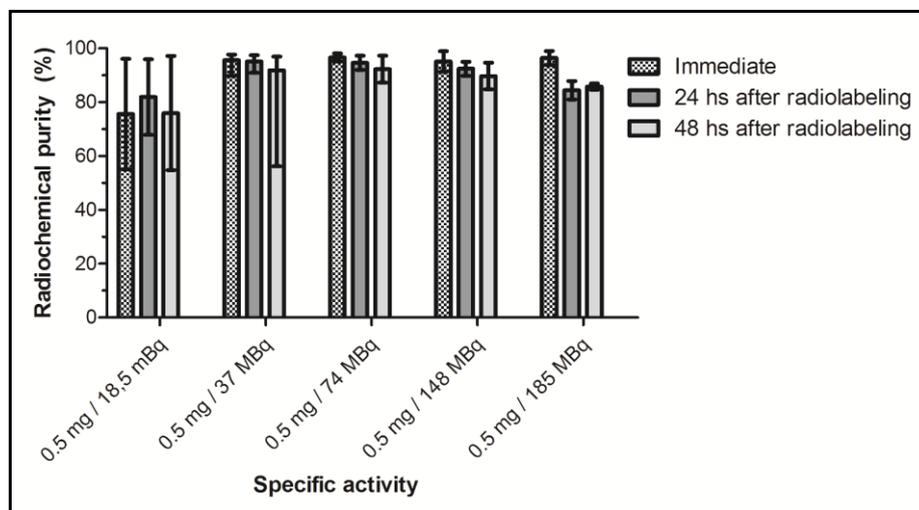
**Figure 3: Radiochemical purity of immunoconjugate radiolabeled in different specific activity (activity variation) for 1 hour at 43 °C, pH 5.5, 350 rpm. Results expressed in median  $\pm$  interquartile with 95% CI ( $n \geq 3$ ).**
