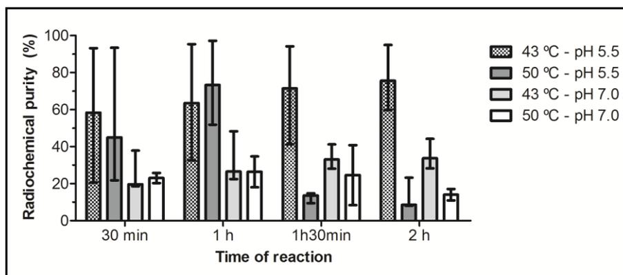
**Figure 4: Radiochemical purity of immunoconjugate radiolabeling in different time, temperature and pH for 0.2 mg of immunoconjugate, 185 MBq (5 mCi) of  $^{177}\text{LuCl}_3$ , 350 rpm. Results expressed in median  $\pm$  interquartile with 95% CI (n = 3).**
