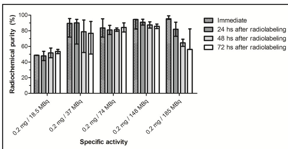
**Figure 3: Radiochemical purity of immunoconjugate radiolabeled in different specific activity (activity variation) for 1 hour at 43 °C, pH 5.5, 350 rpm. Results expressed in median ± interquartile with 95% CI (n ≥ 3).**
