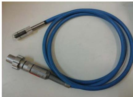
**Figure 2: Ionization chamber PTW 31013**
