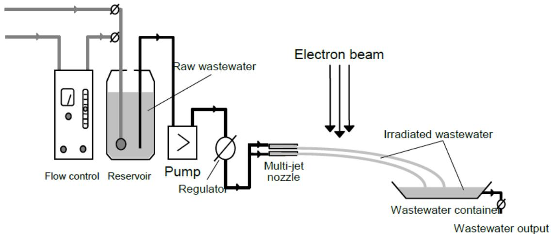
Fig. 1. Laboratory electron beam unit; 50m<sup>3</sup>/day up to 2kGy at continuous operation mode.
