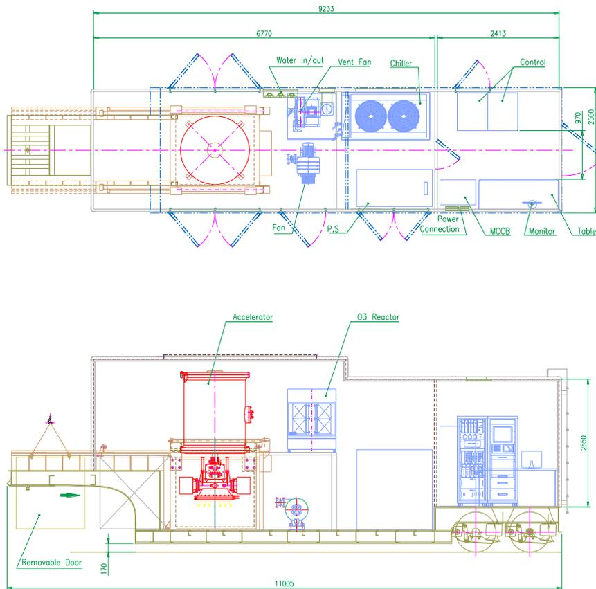
Fig. 3. Mobile Electron Beam Plant (MEB); 500m<sup>3</sup>/day with 2kGy at continuous operation mode.
