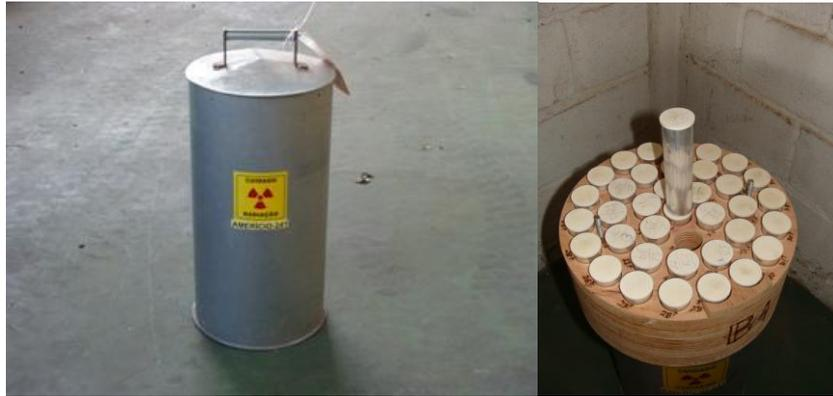
**Figure 3: Packaging storage - left general view and right internal details**
