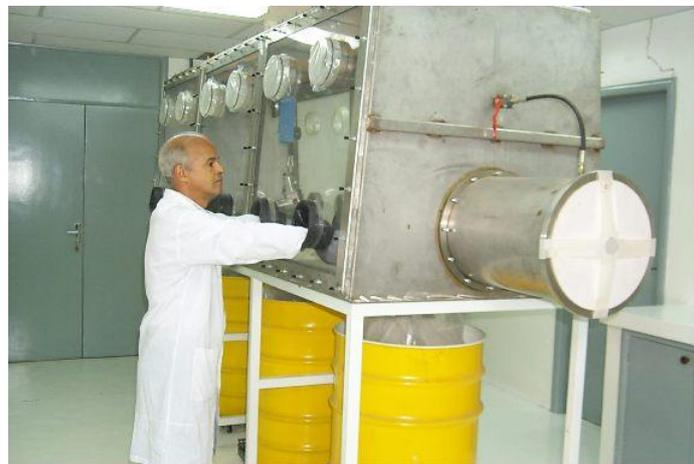
**Figure 2: Glove box for dismantling radioactive lightning rods**
